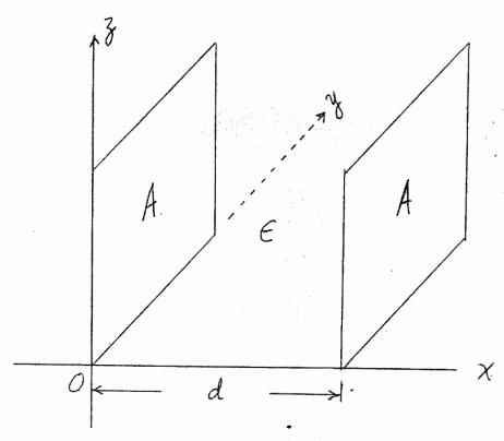
where A is the plate surface area, d is the plate separation and  $\varepsilon$  is the dielectric constant of the insulating material layer in-between the two plates.
