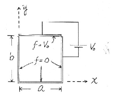
The electric potential in between the two conductors f(x,y) satisfies 2 – D Laplace equation,
