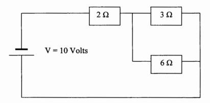
In the circuit drawn above, the battery provides a steady voltage of 10 volts.
