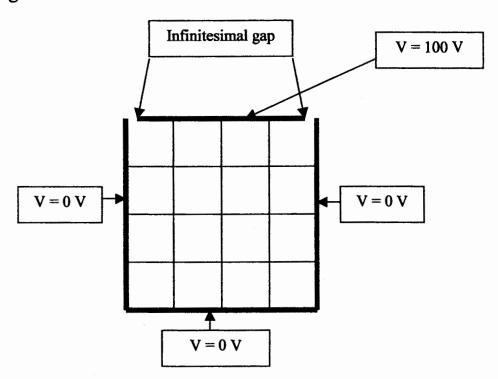
The potential of the top plate is 100 V while the other three conducting plates are at zero potential. Using an iteration method, determine the potentials at the grid points shown in the figure.
