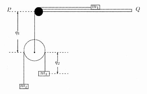
Consider the pulley system shown in Figure above with generalized coordinates  $q_1$  and  $q_2$  as indicated. Assume that the pulleys have negligible masses and that PQ is the reference level. Set up the Lagrangian for the system and prove that Lagrange's equations of motion are given by
