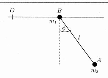
Choosing the generalized coordinates to be x, the distance moved by  $m_1$  from O, and  $\phi$ , the inclination of BA to the vertical,
