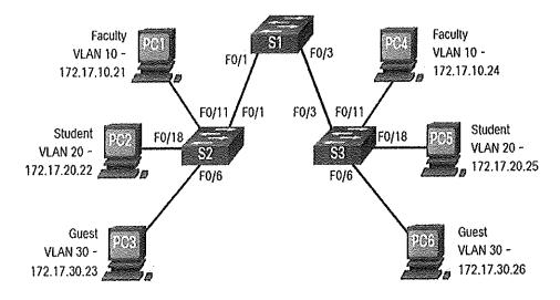
i. Explain how this network can be configured to work as expected, your explanation should also cover the concept of trunking. [15]
