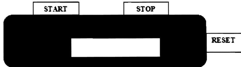
The device has 3 buttons: **Start**, **Stop** and **Reset**. The count value is displayed on the screen labeled count value. The **Start** button starts the counting from zero or from the last count before the counting was stopped. The **Stop** button stops the counting and the display reflects the last value. The **reset** button resets the count value to 0.
