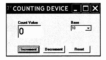
The Increment and Decrement buttons are used to increment and decrement the count value, respectively. The Reset button is used to reset the count to zero. The device can be used to count in different integer modes like base 2, 4, 8 etc. The desired mode or base is chosen using the base selector spin button.
