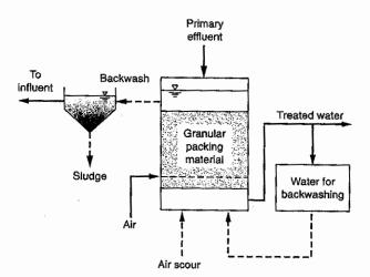
**5E.** Draw a diagram of the activated bio filter and indicate the particular advantage of this set up compared to conventional activated sludge processes.
