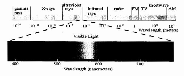
Figure 1: the electromagnetic spectrum. The visible portion of the spectrum is shown in the expanded insert.
