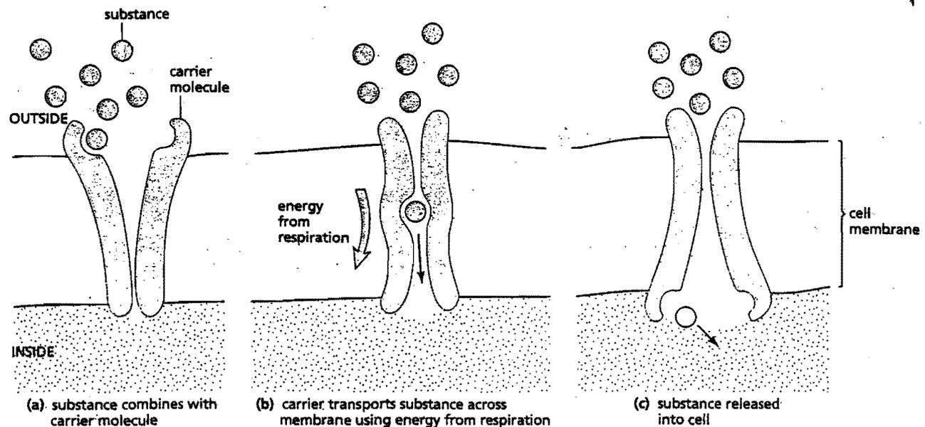
Figure 4.8 Theoretical model to explain active transport
