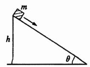
A block of mass m sliding down an incline at constant speed is initially at a height h above the ground as shown in the figure above. The coefficient of kinetic friction between the mass and the incline is  $\mu$ . If the mass continues to slide down the incline at a constant speed, how much energy is dissipated by friction by the time the mass reaches the bottom of the incline? [10 marks]
