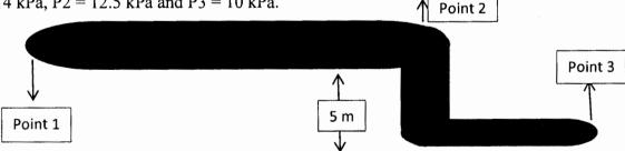
If the diameter of the pipe at point 1 is equal to the diameter at point 2 and it is 60 mm and that at point 3 is 40 mm;
