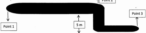
If the diameter of the pipe at point 1 is equal to the diameter at point 2 and it is 60 mm and that at point 3 is 40 mm;
