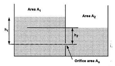
i. Determine the *ideal velocity* at point 2 (at the centre of the orifice).
